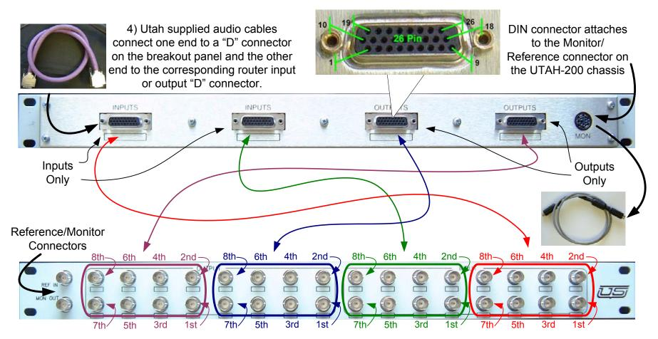
Note: The numbering on each set of eight BNC's indicate which input or output the BNC is connected too. For example: If the far right (red) set of eight were connected to the "D" connector on the router for inputs 00 to 07, the BNC labeled "1<sup>st</sup>" would be connected to Input 00, "2<sup>nd</sup>" would be input 01 and so forth.
